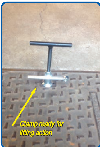
Engagement of the lever in the clamp
